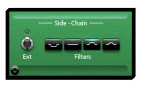
Some of the most respected 'classic' compressors actually filter the side-chain [the signal used to drive the gain element], in order to weight the compression in such a way as to be triggered by a particular frequency range. The weighting of the side-chain filter will affect the character of the compressor, although the saturation and transient characteristics of this filter are an important factor too.
