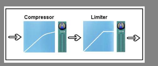
This is an important distinction to understand, as it is very different to a simpler 'all in one' compressor/limiter. By implementing the limiter as a separate process, independent control is maintained over all attack/ release times, and the compressor may affect the signal even when the limiter threshold is lower than the compressor threshold.
